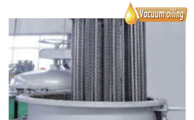
▲ Through the vacuum pump, each aperture of parts is filled with wear-resistant grease and the chain life is extended by 30%.
