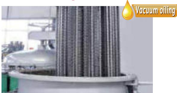
A vacuum pump is used to extract air from the oiling container, so that the air inside the chain parts is drawn out, forming a negative pressure, and filling the gaps of the parts with wear-resistant grease. This technology makes the chain oil evenly and fully, good lubrication, improves the wear resistance of the chain, and extends the life by more than 30%
